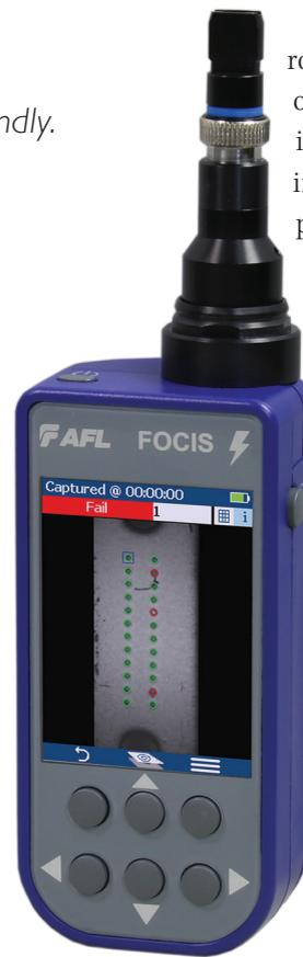
The FOCIS Lightning MPO fiber inspection system from AFL takes about one second to test a fiber end. It also offers a composite view of the entire endface.
